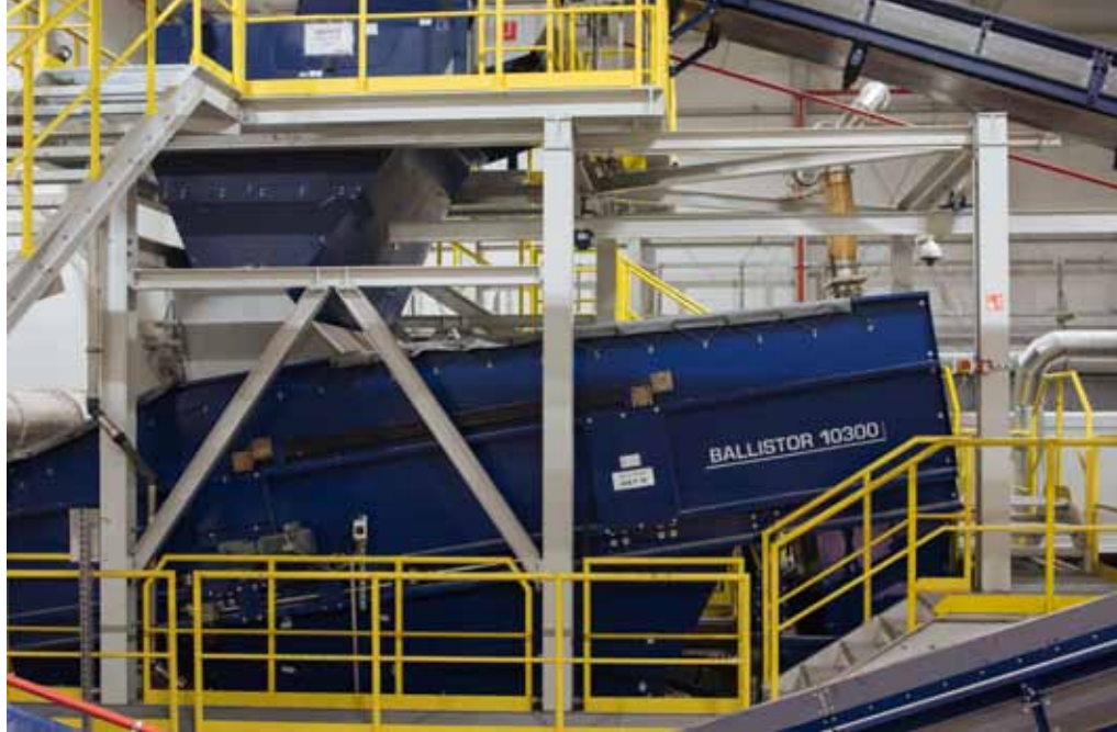
The Ballistor separates the high caloric fraction from the waste stream.
