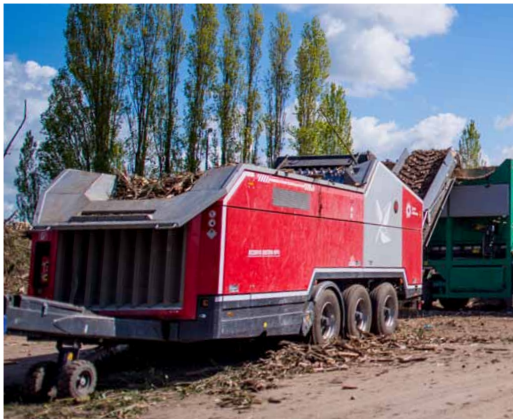
The right technology can turn even low-grade input material into high-grade fuel: shredding with the Axtor, screening with the Multistar L3 and removal of plastic and stones with the Hurrifex.
