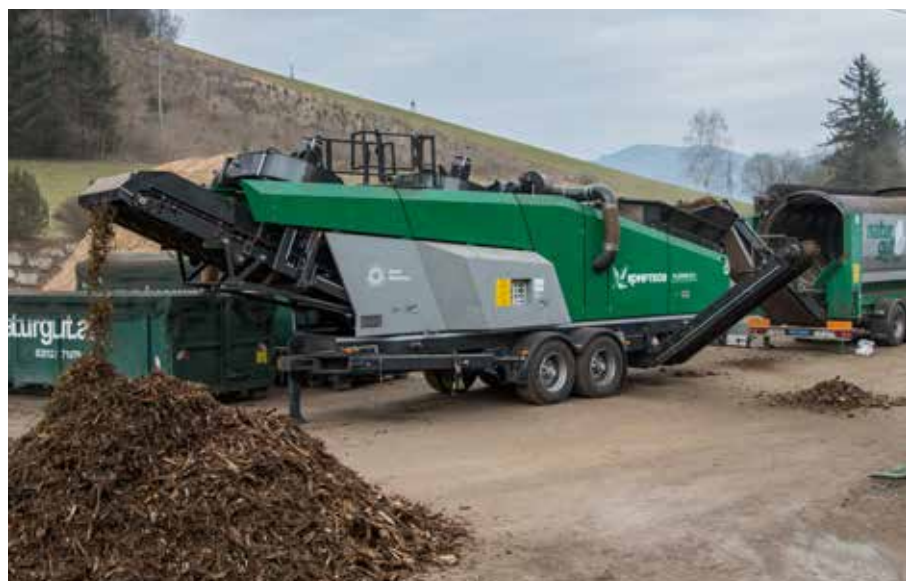
Contraries are a big problem in compost. With the Hurrifex heavy objects like stones as well as light materials like plastics can be removed in a single pass.
