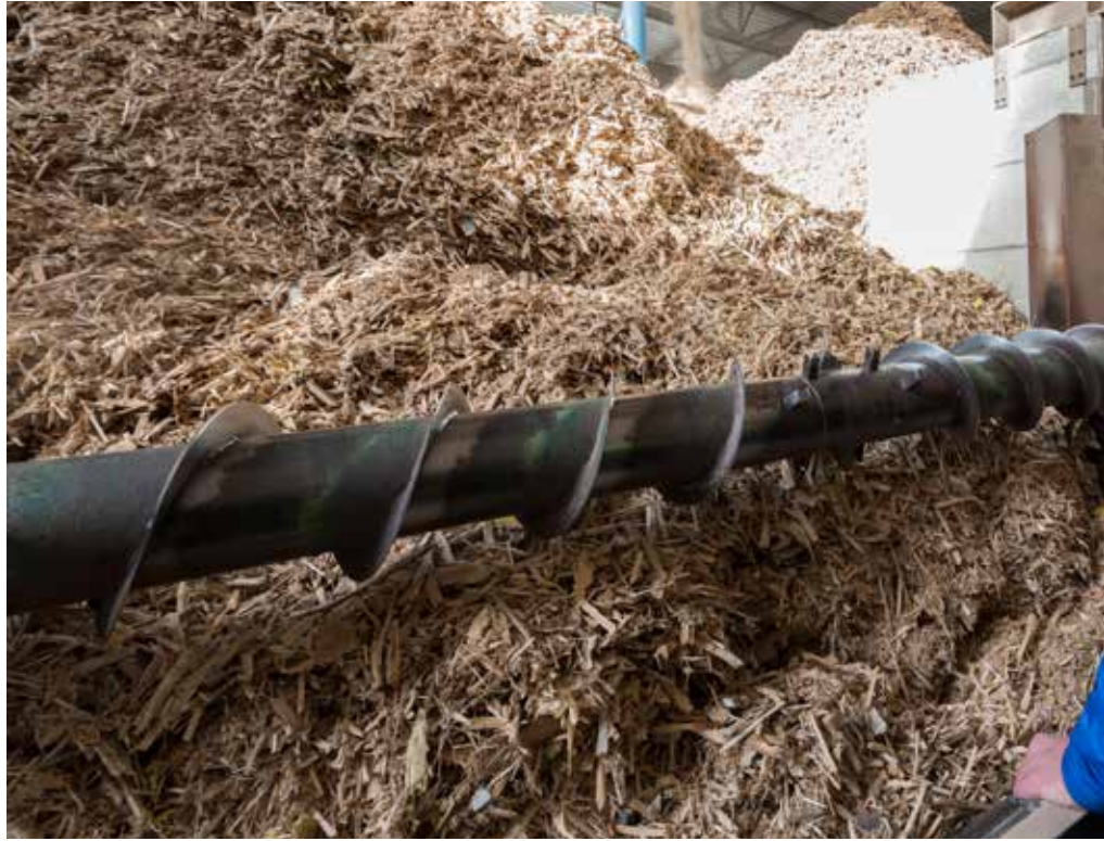
Andreas Suter inspects the fill level of the intermediate bunker. Fuel goes from here to the burner.
