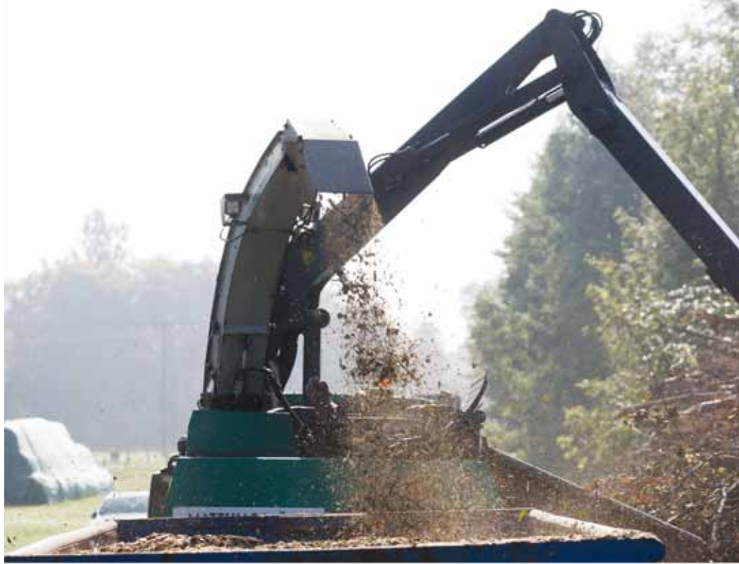
Discharge is by fan or a separate discharge conveyor.
