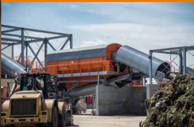
The new processing line with Komptech drum screen.
