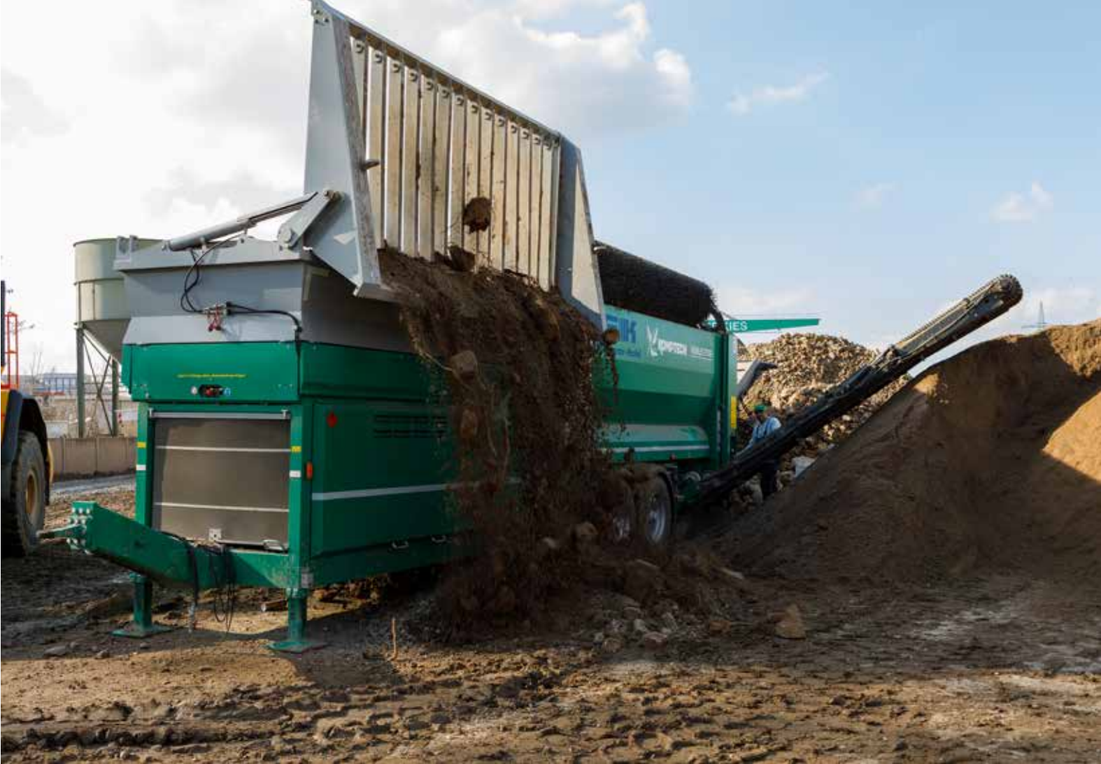
The hopper pre-screen separates out larger items in the input.
