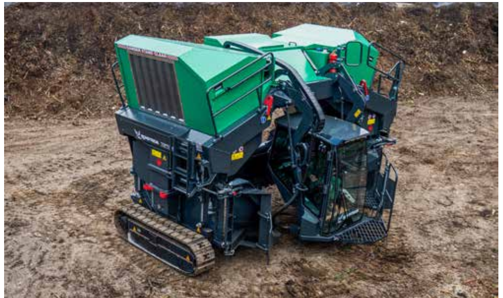
When the cab is in the transport position the turner is very compact, simplifying multi-site use.
