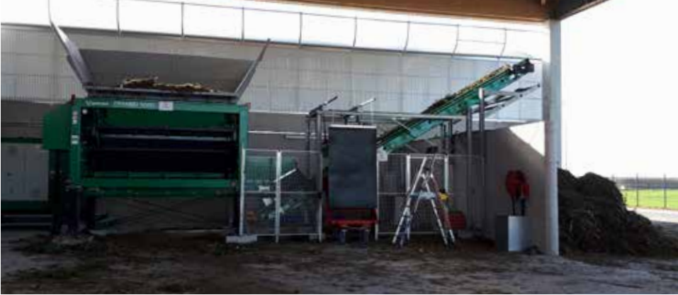
Stage 1 – Shredding: A Crambo 5000SE equipped with a biobasket XL shreds the input. Ferrous metal is removed by an overband magnet.
