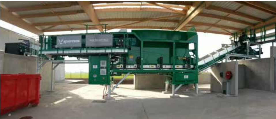
Stage 3 – Screening: This step is carried out by a Multistar XL SE star screen to extract two wood fractions and the compost in a single pass.
