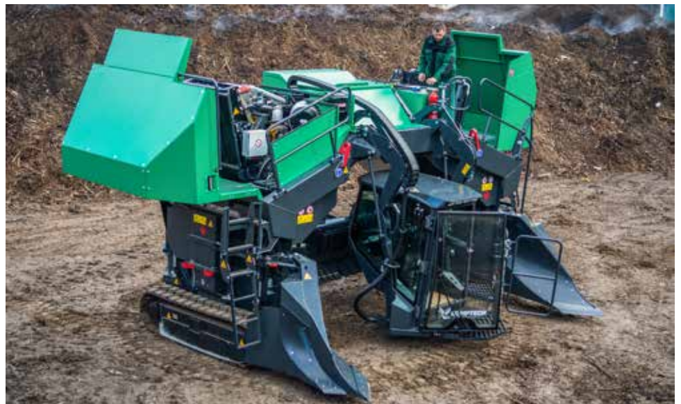
A press of a button turns the left and right body panels into roomy maintenance platforms.
