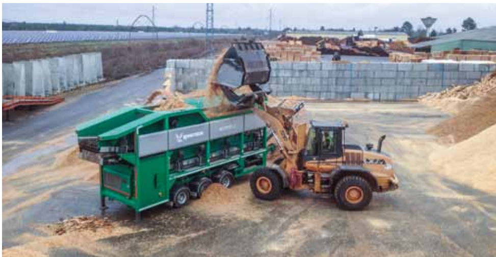
Two Multistar L3 star screens clean up the fuel.
