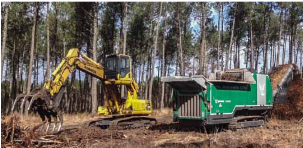
Clean rootstocks are ready for chipping with the Axtor.
